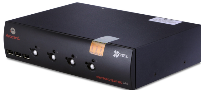
The SC 300 series switch is available in 2, 4 and 8 port configurations
