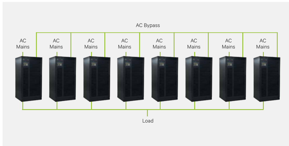
Liebert® EXL™ distributed parallel configuration, with 8 UPS units in parallel
