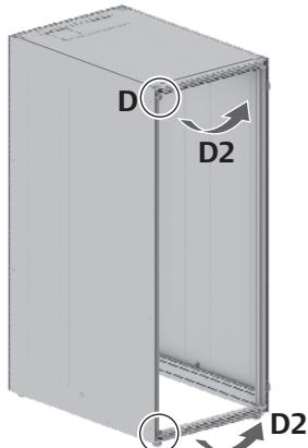
Reverse the locking plates on the base frame
