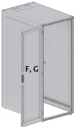
**Remove the handle and the swing-lever**
