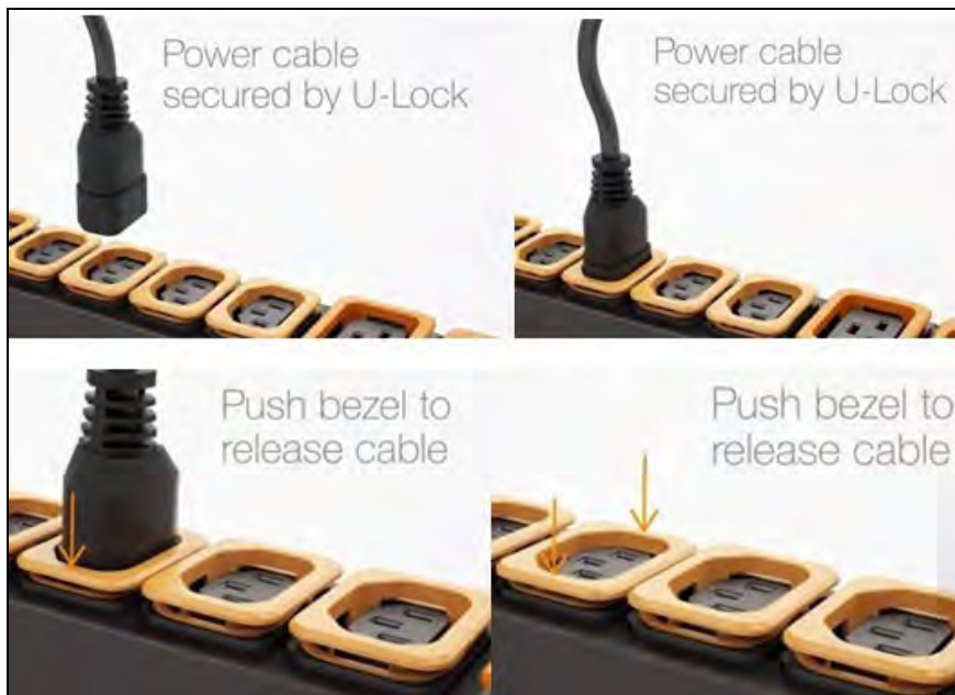
Figure 3.3 U-Lock Cord Retention Operation
