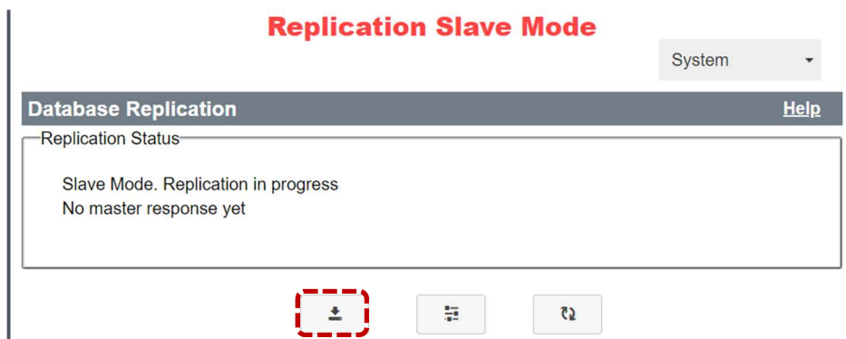
Figure 5-120 Slave Unit Management Interface Homepage&gt;Download Master Backup
