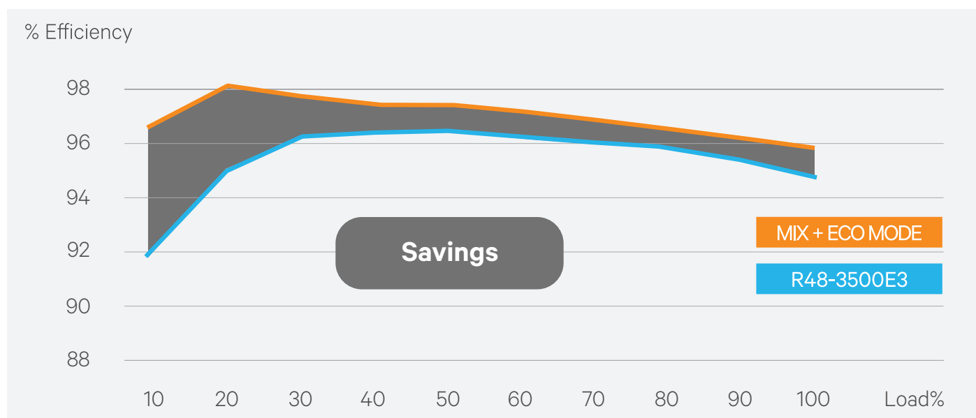
Figure 4: Upgrading 96% Rectifiers to 50-50 Mix (96% + 98%) with ECO Mode Activated
