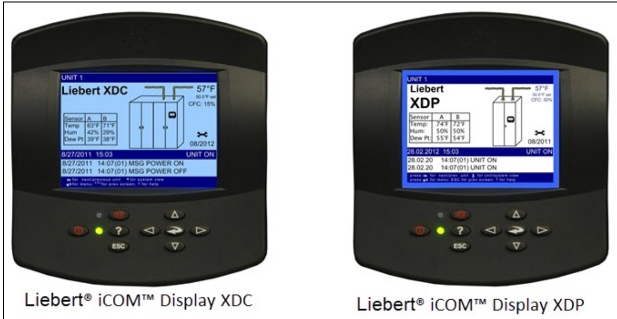
Figure 7.1 Liebert® iCOM™ Display—Liebert® XDC and XDP
