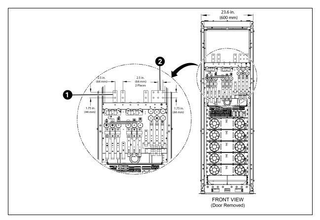
Figure 4.7 Ground and Neutral Busbar Connections - 20-100 kVA Frame Busbars
